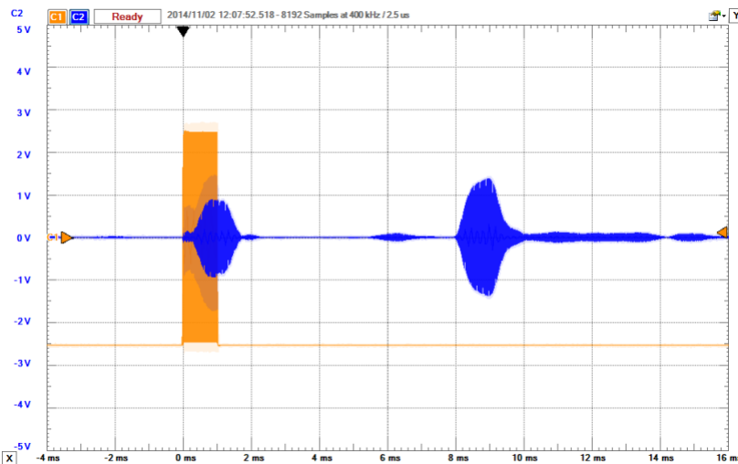
Figure 5: Sample data. The orange is the transmit signal and the blue is the received. In this case there is about 8 ms between transmitted and received signal, indicating the pulse traveled about 9 ft, or the wall is 4.5 feet away.
