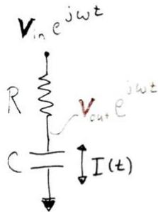
$$\frac{V_{out}}{V_{in}} = \frac{1}{1 + j\omega RC}$$
