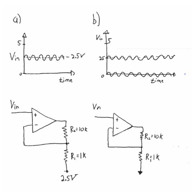
Figure 1: Amplifier circuit with 2.5 and ground reference
