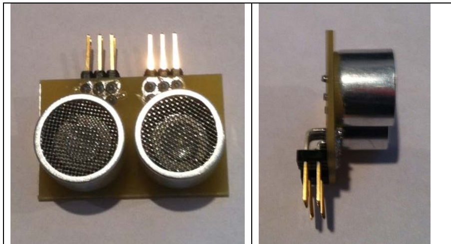
Figure 2: The transducer board for the ultrasound experiment. The transmitter and receiver are the same. The gap in the pins on the lefthand picture should straddle the middle break of your breadboard. On the right hand picture, the pins on one row should be connected to ground and the other row to either the output of the transmitter or the input of the receiver. The transducers have no preferred electrical orientation.
