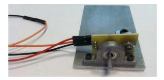
While watching the Scope screen, move the axle of the device around by hand. If everything is working, you should see the voltage change as you adjust the angle. The voltage should vary between 0 and 5 volts. You will need to adjust the x and y axis settings. On the right of the Scope screen, turn off channel 2, adjust the time scale to be something like 1 second per division and the Channel 1 range to be 1 volt per division.
