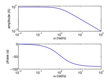
FIG. 2 Low pass filter. Relative amplitude as a function of frequency and the phase angle in degrees as a function of frequency when RC = 1.
