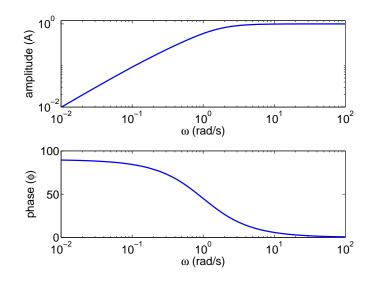
FIG. 4 High pass filter. Relative amplitude as a function of frequency and the phase angle in degrees as a function of frequency when RC = 1.
