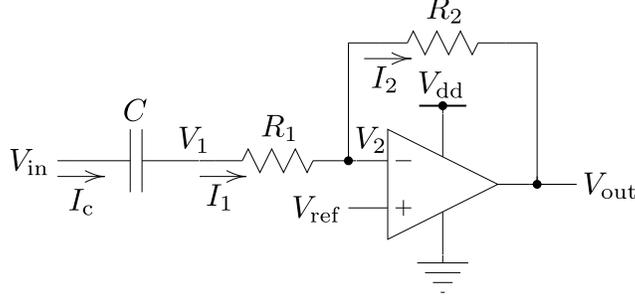
**Figure 9:** Schematic of a first-order high-pass filter/amplifier circuit. The filter's time constant is given by  $\tau = R_1 C$ , its corner frequency is given by  $\omega_c = 1/\tau$ , and its pass-band gain is given by  $A = -R_2/R_1$ .
