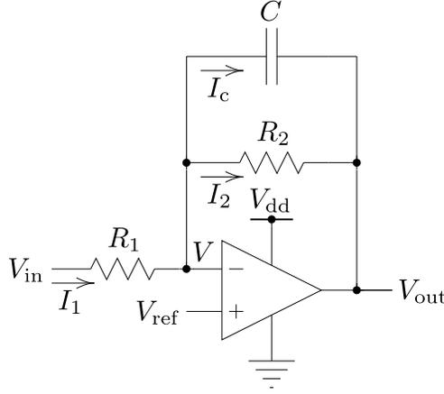
**Figure 8:** Schematic of a first-order low-pass filter/amplifier circuit. The filter's time constant is given by  $\tau = R_2C$ , its corner frequency is given by  $\omega_c = 1/\tau$ , and its pass-band gain is given by  $A = -R_2/R_1$ .
