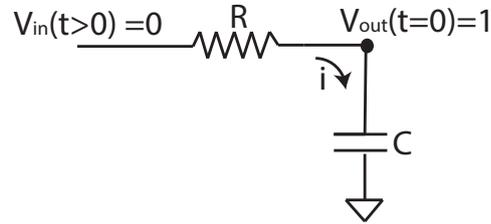
FIG. 1 Circuit that we will analyze. Initially the voltages are set to 1 and then suddenly the input voltage is pulled down to zero.
