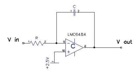
To see that this circuit integrates, just use all our laws for the resistor, capacitor, and op-amp.
