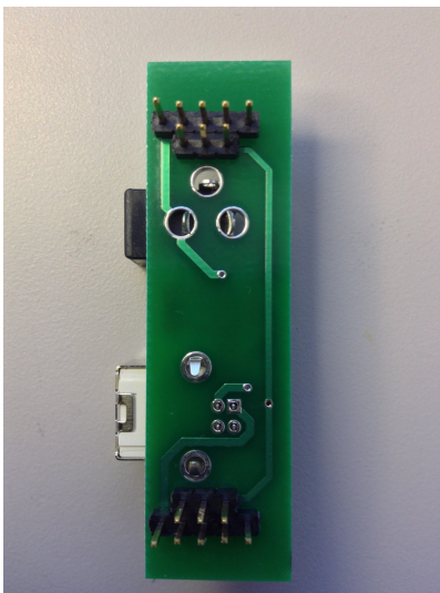
Insert the USB and the barrel jack connectors. Flip the PCB over.
